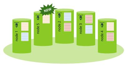
Movement is decomposed into adding a replica followed by removing a replica
