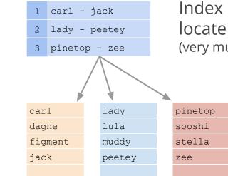
Index structure used to locate ranges (very much like a B-tree)
