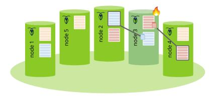
The leaseholder can send commands to be replayed OR it can send a snapshot of the current Range data. We apply heuristics to decide which is most efficient for a given failure.
