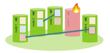
The failed replica is removed from the Raft group and a new replica created. The leaseholder sends a snapshot of the Range's state to bring the new replica up to date.
